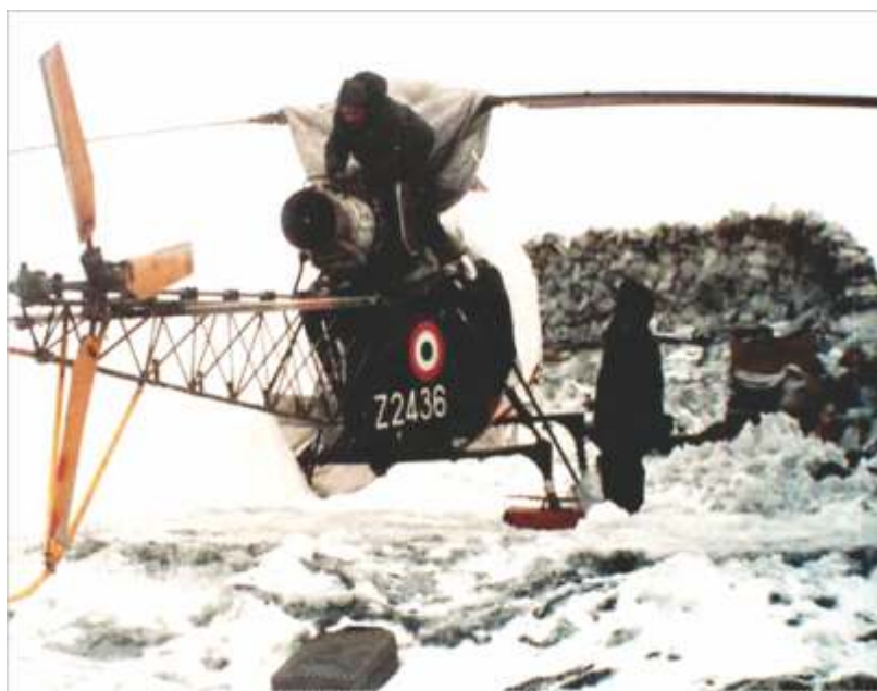
The unserviceable Cheetah helicopter at Amar, Siachen, whose engine was changed at night - using kerosene lamps and torches
